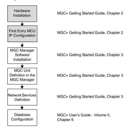
Figure 2-1: Installation and Configuration Workflow - Hardware Installation
